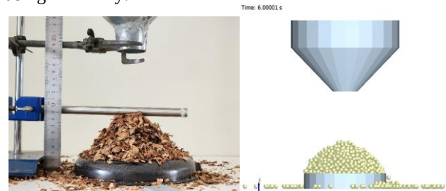
Fig. 3. AoR (a) experimental test (b) EDEM simulation
