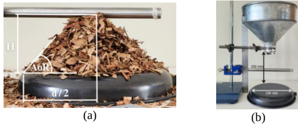
Fig. 2. AoR (a) measurement theory (b) experimental setup
